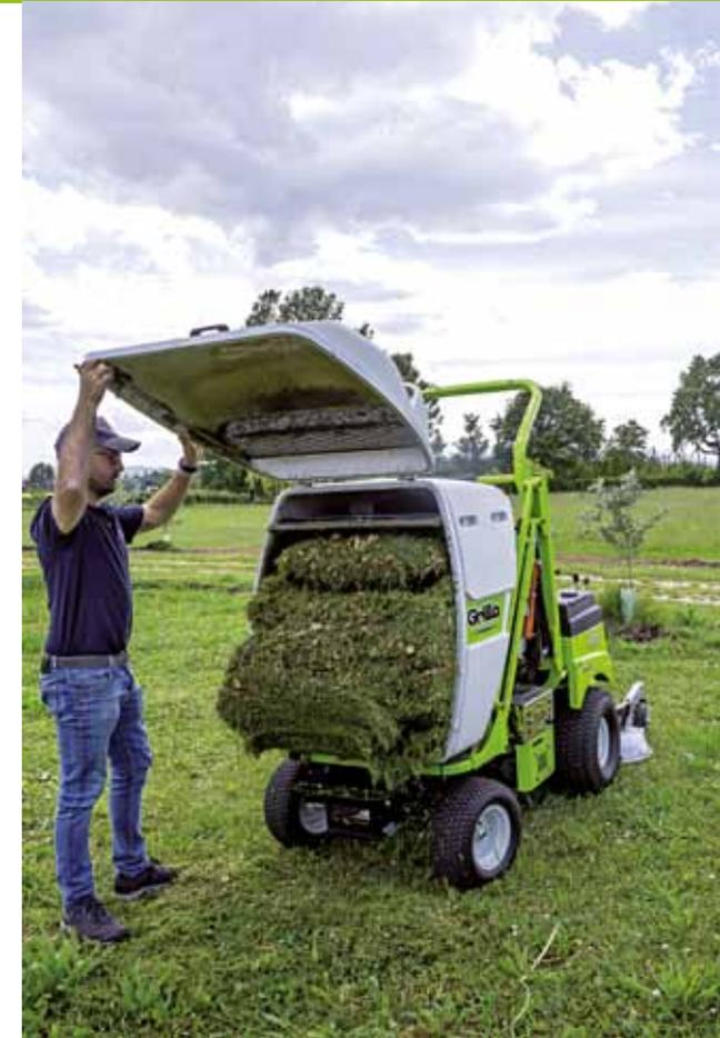
The hydraulic services for raising and tipping the grass collector are operated from the driver's seat by means of convenient levers that make grass discharge and return to the working position extremely smooth and fast. A third lever is used to hydraulically raise the deck for easy movement over kerbstones and obstacles.
