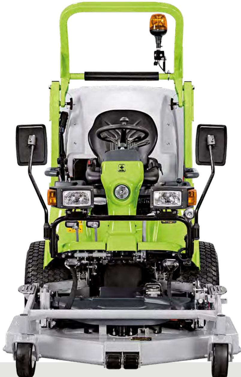
The FD 900 is equipped with a Yanmar 3TNV80F diesel engine, 25 HP, three cylinders, compliant with the directives EC (NRMN) STAGE V (EUROPE) and EPA FINAL TIER 4 (USA), mounted on shock-absorbers into a very robust frame, designed to protect the machine main components.
