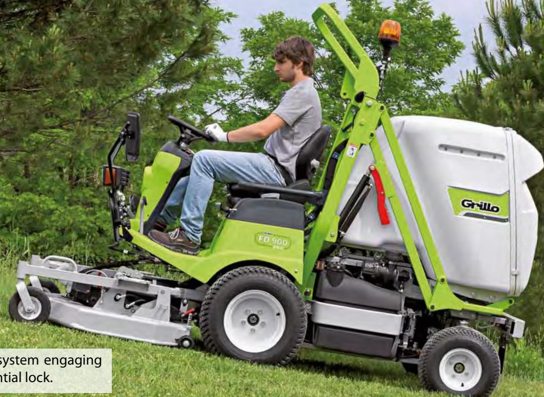
The innovative permanent 4WD ensures, via the hydraulic differential, **maximum grip under all working conditions and even on tight turns without damaging the grass.** Perfect weight distribution combined with the automatic and/or manual differential lock make this mower safe and steady when cutting on slopes.
