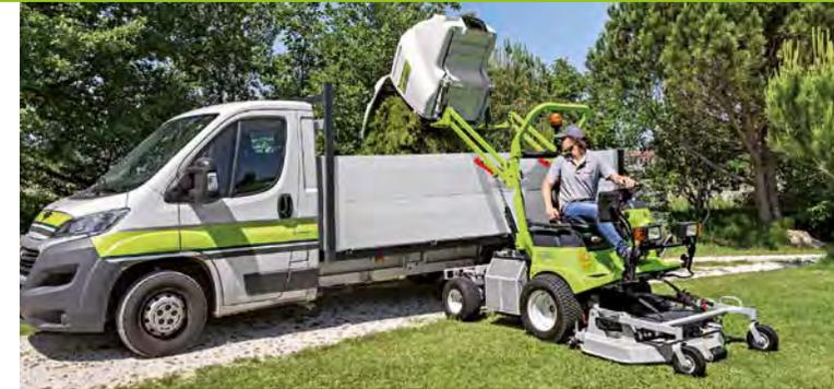
The hydraulic services of both the grass-catcher and cutting deck are activated via practical levers fitted with safety system devices and are located on the dashboard. It is very easy and quick to empty grass into a truck and also easy to raise the cutting deck when negotiating obstacles or kerbs.
