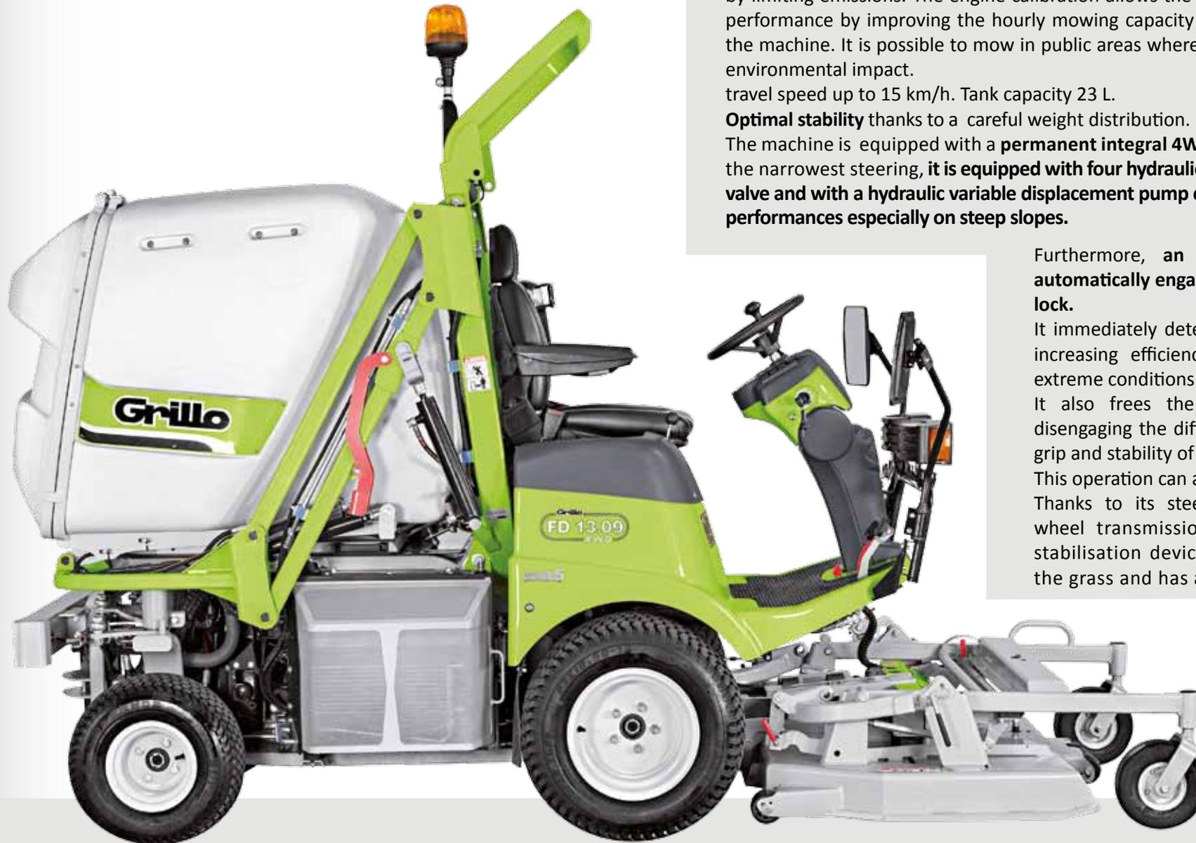
The latest **3TNV82A STAGE 5 1331 cc diesel engine (26 HP, 2800 rpm)** liquid cooled with electric fan and both automatic and manual cleaning, protects the environment and health by limiting emissions. The engine calibration allows the optimisation of consumption and performance by improving the hourly mowing capacity and the return on investment of the machine. It is possible to mow in public areas where specific norms require to reduce environmental impact.
