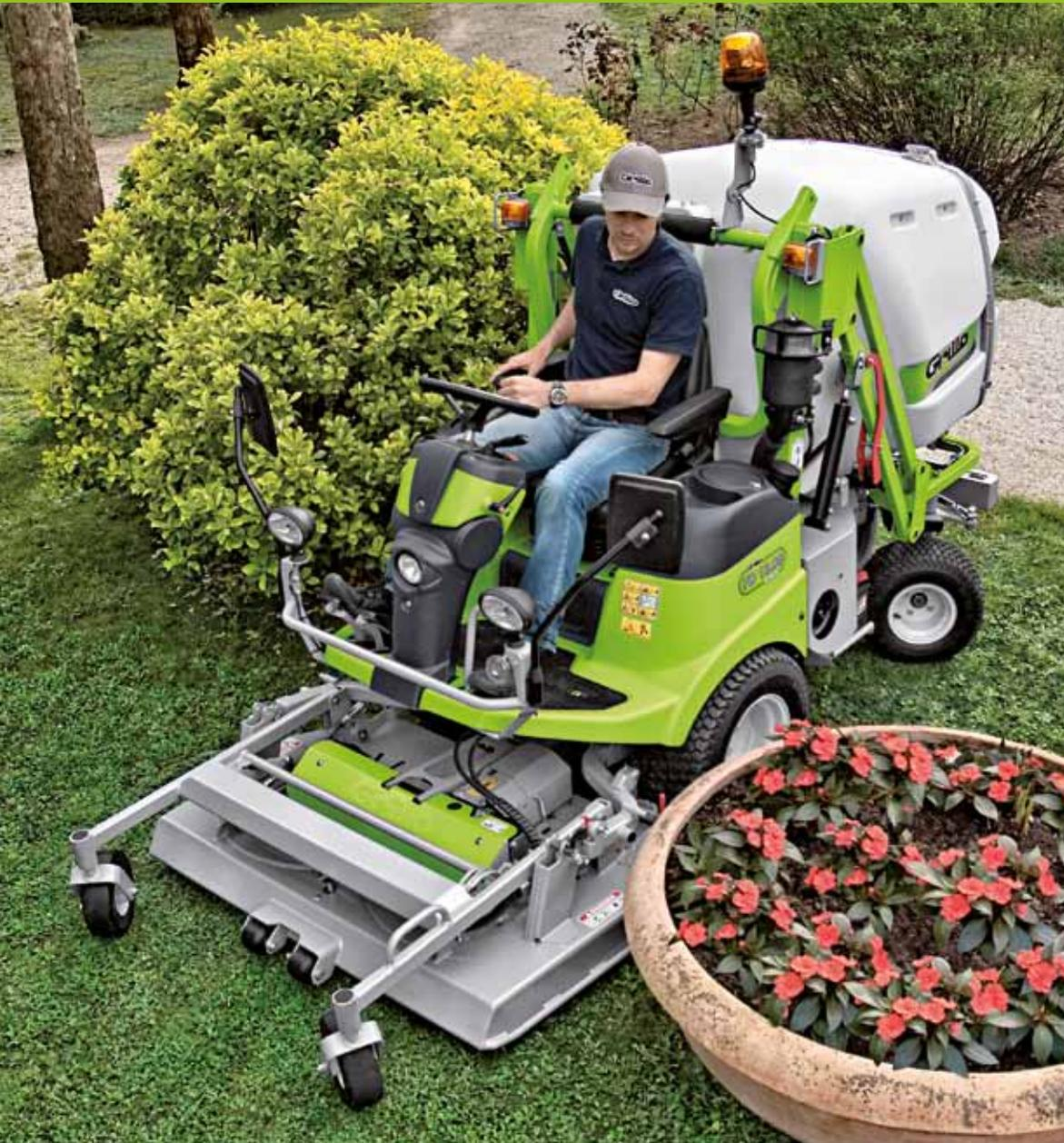
The **FD 13.09** is a compact mower with a very narrow wheelbase, **equipped with power steering and a turning radius of only 31 cm.**
