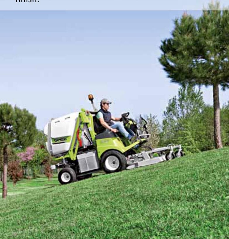
The **integral permanent 4WD** system allows users to work in excellent **safety conditions on any slope**.
