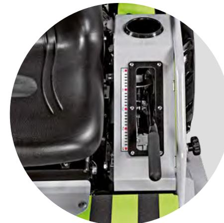
The cutting height adjustment is progressive and assisted via a balanced lever with automatic locking in any position. The cutting deck locks automatically when the lever is released.
