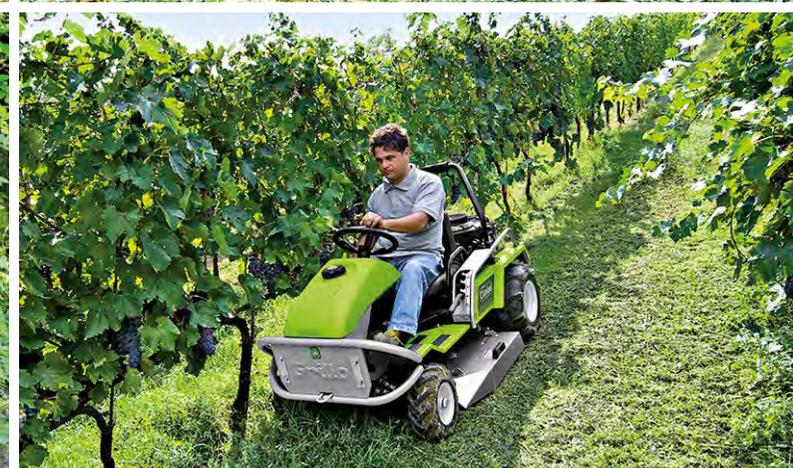
The extremely small **turning radius** of only 38 cm allows to move in tight areas.
