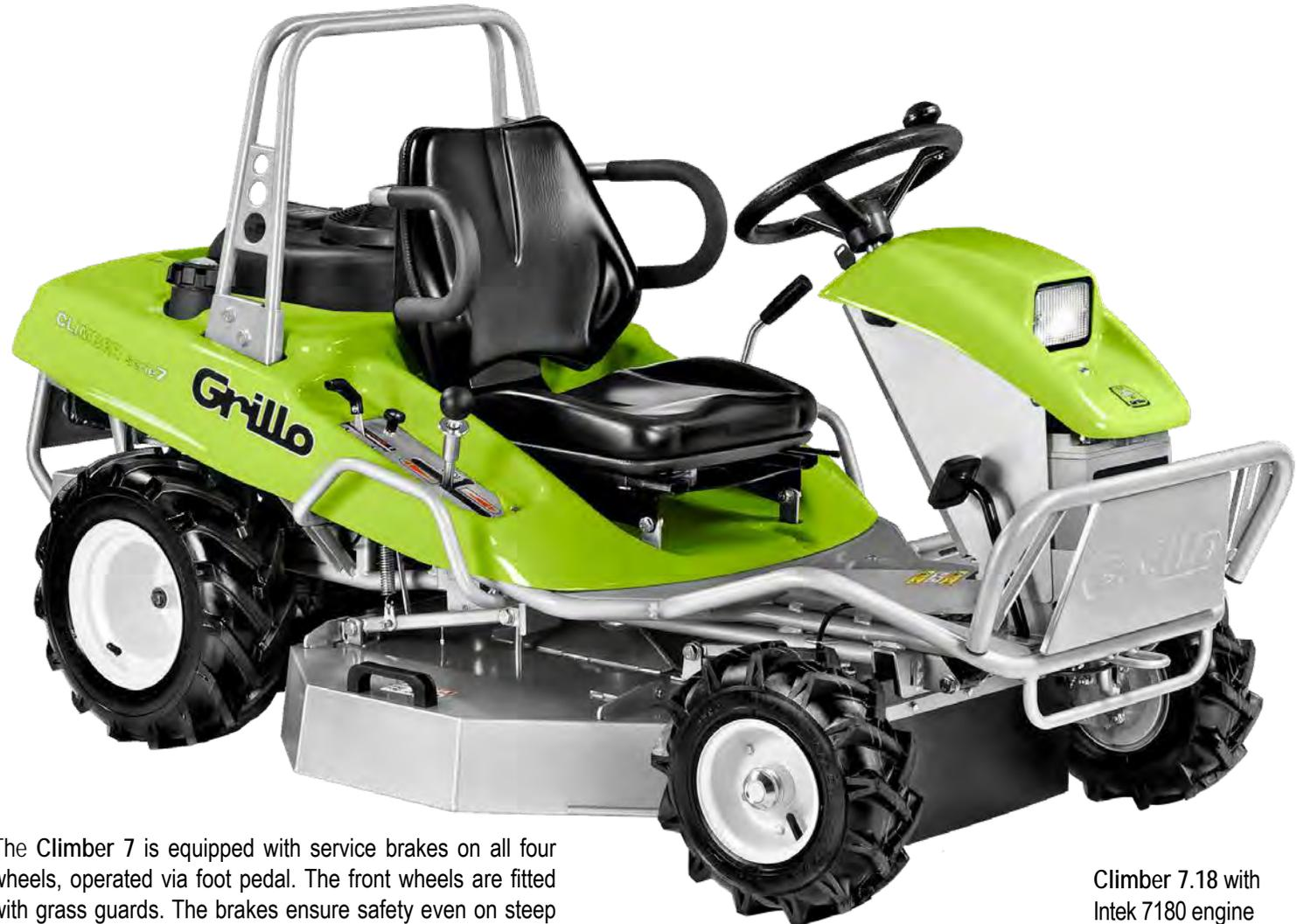
The Climber 7 is equipped with service brakes on all four wheels, operated via foot pedal. The front wheels are fitted with grass guards. The brakes ensure safety even on steep slopes and slippery terrain.
