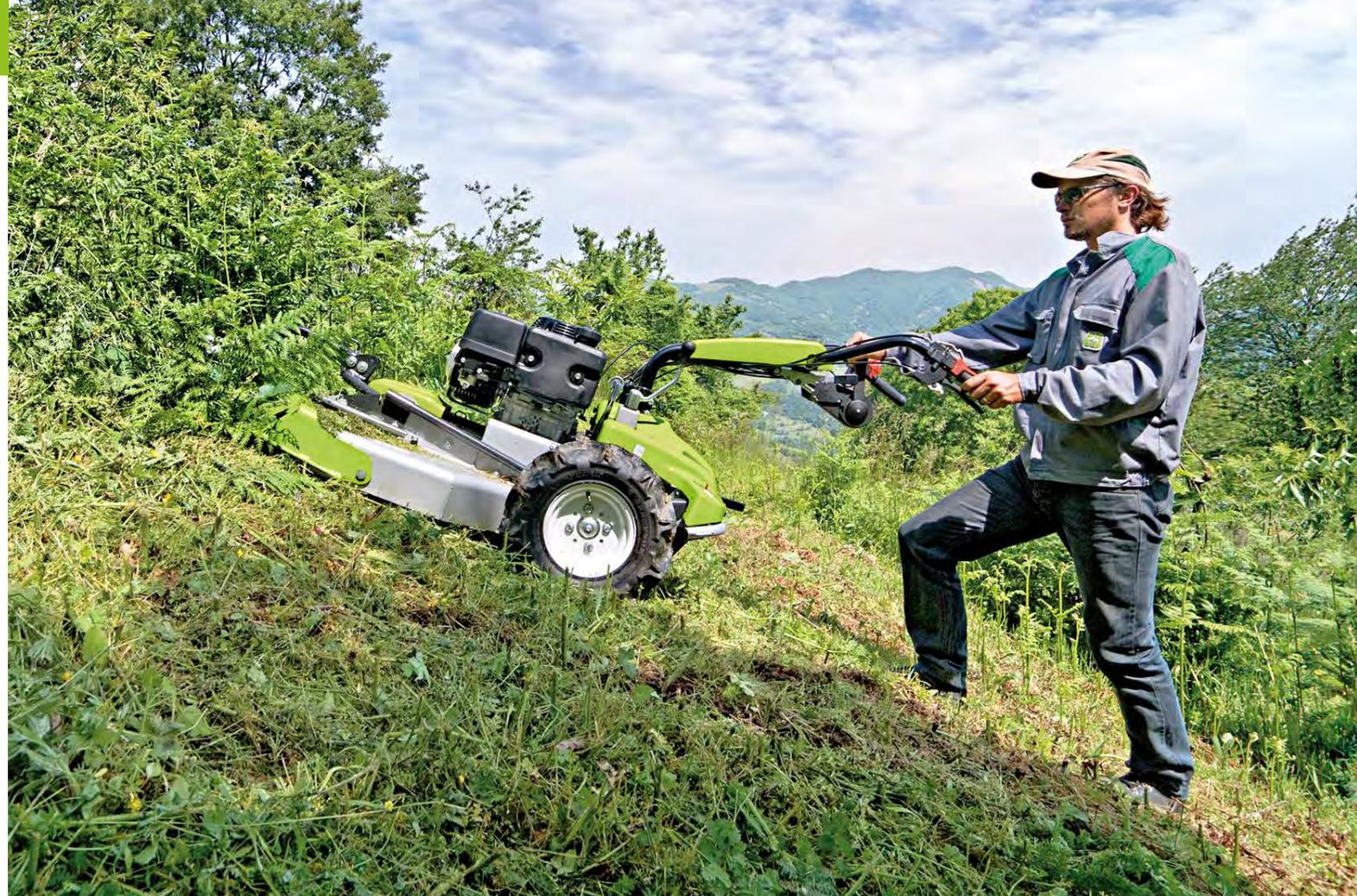
The maximum cutting height of 15 cm is ideal when the terrain is very uneven to avoid accidentally hitting the ground.
