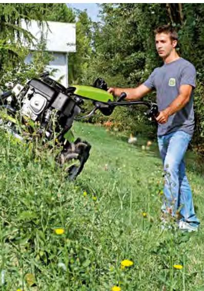
The front wheel can be locked for hillside cutting, making work much easier. Furthermore, the engine is equipped with a forced lubrication pump, which allows work on steep slopes without damaging the engine.
