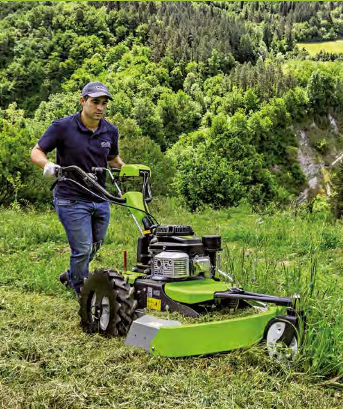
The CL 62M is fitted with a OHV single cylinder petrol engine, 179 cc, 4.5 HP with a 1.6 L fuel tank and forced lubrication system, allowing the machine to work on slopes up to 30°.
