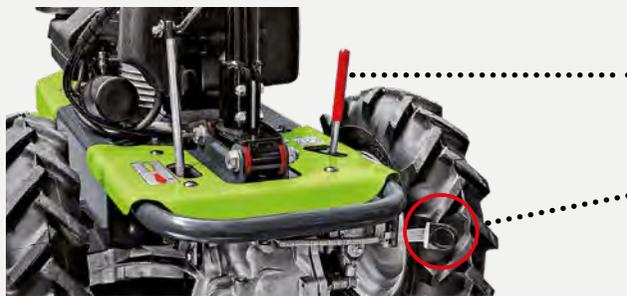
The machine has a **disc parking brake** that keeps the machine stationary even on a slope.
