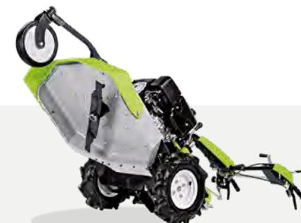
The CL 75 can be easily positioned vertically by simply resting the handlebar on the ground. This makes **maintenance and cleaning** of the cutting deck very easy.
