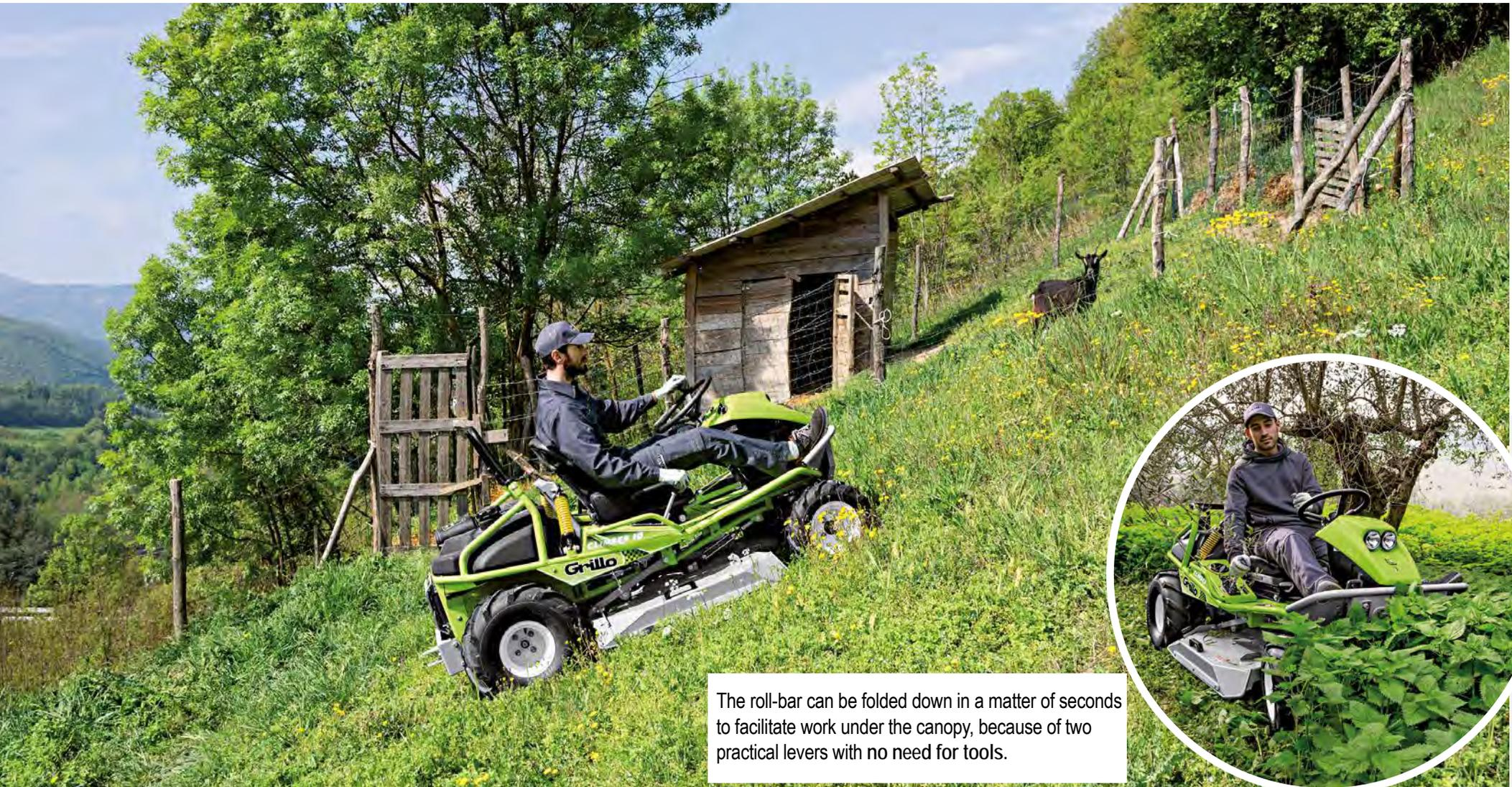
The roll-bar can be folded down in a matter of seconds to facilitate work under the canopy, because of two practical levers with no need for tools.
